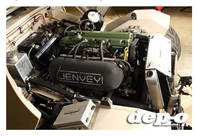
The chassis has been strengthened, a thoroughly rabid 191bhp 1796cc throttle-bodied K-series has been fitted along with a five-speed gearbox and LSD. The drum brakes have been replaced by discs and alloy billet calipers, the suspension lowered and converted to telescopic dampers, double front wishbones and the rear benefits from Frontline's clever Rear Traction Link.
